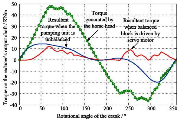
Fig. 4. Torque on the Reducer's Output Shaft
