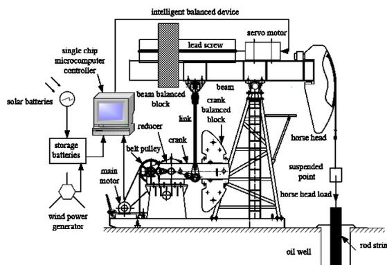
Fig. 1. Whole Structure of the Intelligent Balanced Device
